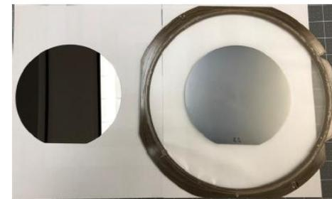
150 mm wafer (60  $\mu\text{m}$  thick) debonded
